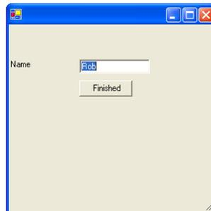
However at the moment nothing happens when the button goes down. To get this to work we have to bind a method in our program to the event which is generated when the button is pressed. The windows forms system uses *delegates* to manage this.
